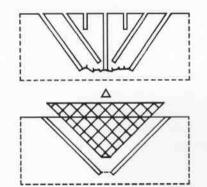
Trenching in sedimentary rock or concrete not reinforced
