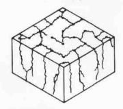
Concrete foundation, free standing, slightly reinforced. Holes must be drilled inside the reinforcing steel.
